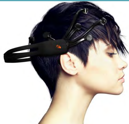
Emotiv Epoc headset, detecting conscious thoughts, emotions, facial expressions and head rotation
